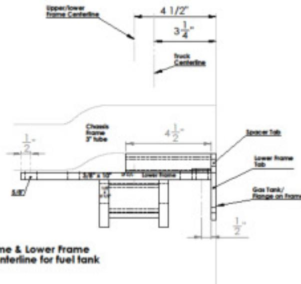
Note: Entire scissor Upper Frame & Lower Frame are offset 1 1/4" from truck centerline for fuel tank clearance.
