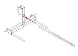
Insert Bale spear (D) into designated collar attaching with 1/2 x 3" bolt, flat washer, and Nut.
