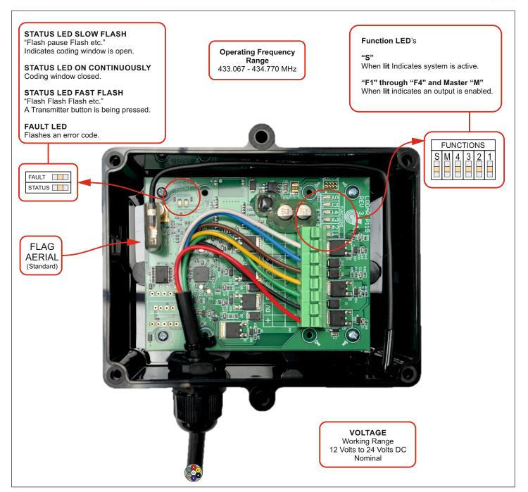
**Fault Codes** - Number of flashes indicate Fault Code. "1 = Flash Pause, 2 = Flash, Flash, Pause, etc"
