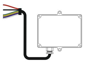
Secure using 5mm (3/16") bolts (not supplied) through the 2 mounting feet
